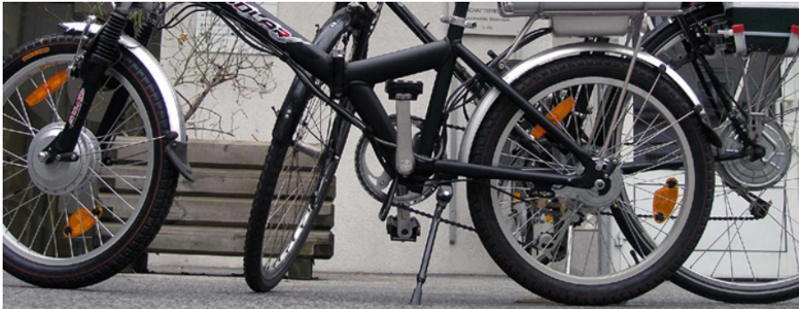
FIGURE 5.45 Bicycle side reflectors. Photo: No machine-readable author provided. Gerfried assumed (based on copyright claims). [GFDL ( http://www.gnu.org/copyleft/fdl.html ), CC-BY-SA-3.0 ( http://creativecommons.org/licenses/by-sa/3.0/ ) or CC BY-SA 2.5-2.0-1.0 ( http://creativecommons.org/licenses/by-sa/2.5-2.0-1.0/ )], via Wikimedia Commons. https://upload.wikimedia.org/wikipedia/commons/9/94/Hyperbikes.jpg .
